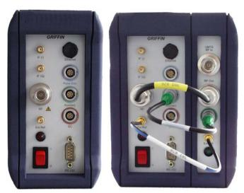
The 8300 Series Griffin consists of the measurement receiver, an optional up or down converter, and the Griffin Front Panel Software to operate the instrument from a PC.
