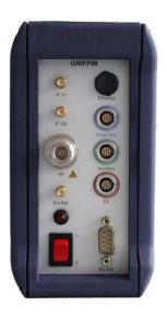
**Antenna input** The antenna should be chosen to suit the frequency band of the Griffin in use (800 to 1000 MHz or 1700 to 2000 MHz). It can be connected directly to the RF input connector or via a length of lowloss cable. The input is a conventional 50 W N-type.
